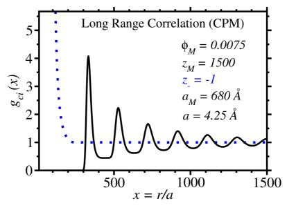
Macroion-macroion (solid line) and macroion-counterion (dotted line) radial distribution functions for a macroions dispersion of diameter  $a_M = 160a$ , in the absence of salt, as a function of the distance of the central macroion, measured in little ions diameter size, a.  $\phi_M$  is the colloidal volume fraction,  $Z_M$  and z- are the macroion and counterion valences. Notice that  $r = xa = 1500a \approx 6,400$  Å.
